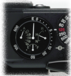
The needle indicators on the R-D1
