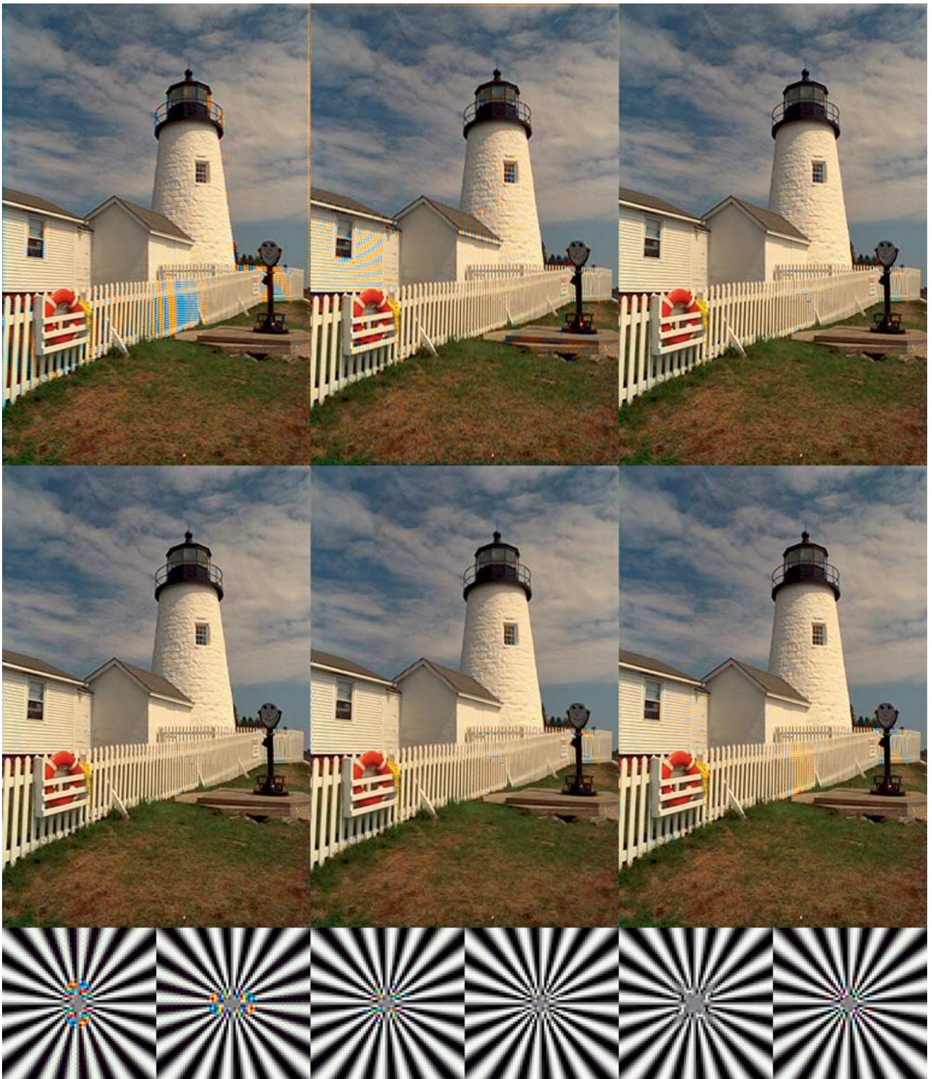
Fig. 10. Example outputs using “lighthouse” and “ray” images. From top to bottom, left to right: horizontal interpolation ( f_H ), vertical interpolation ( f_V ), directionality selection output ( f ), interpolation artifact removal (final output), and proposed method with forced h_{0=0} (see text) method [8].
