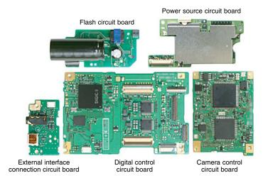
To make the camera smaller, the external interface connection circuit board has been separated from the digital control board and both sides are used. It has the USB port (MINI B), conforming to USB 2.0 Hi-Speed, and the video OUT terminal.
